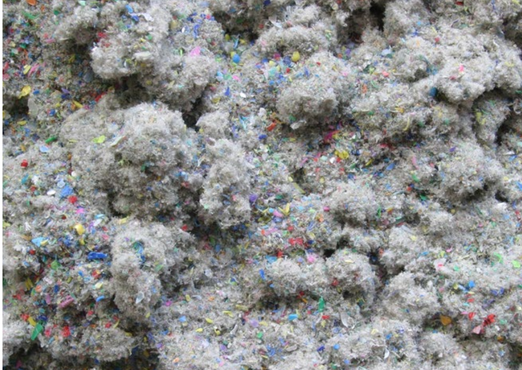
Defibred Paper and Dirt removed in the Dry Cleaner
