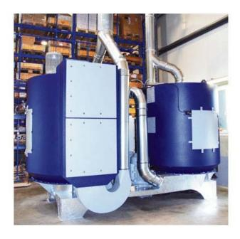
DRD 18 model. The DRD 26, with a centrifugal diameter of 2,600mm, replaces the DRD 24. Both new models are available in single- and two-stage versions.
