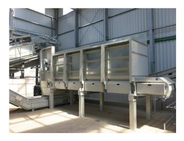
Designed for smaller feed volumes, the innovative **Multi**Feeder handles storage capacities from 10 to 47m<sup>3</sup>.
