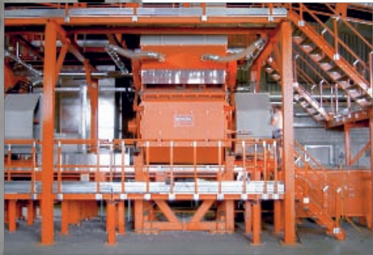
Core of the plant: the FineCut secondary shredder.
