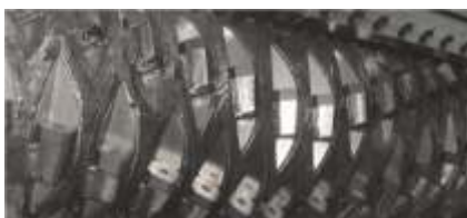
Minimum wear: the PowerLine rotor with blades that can be reversed a number of times.
