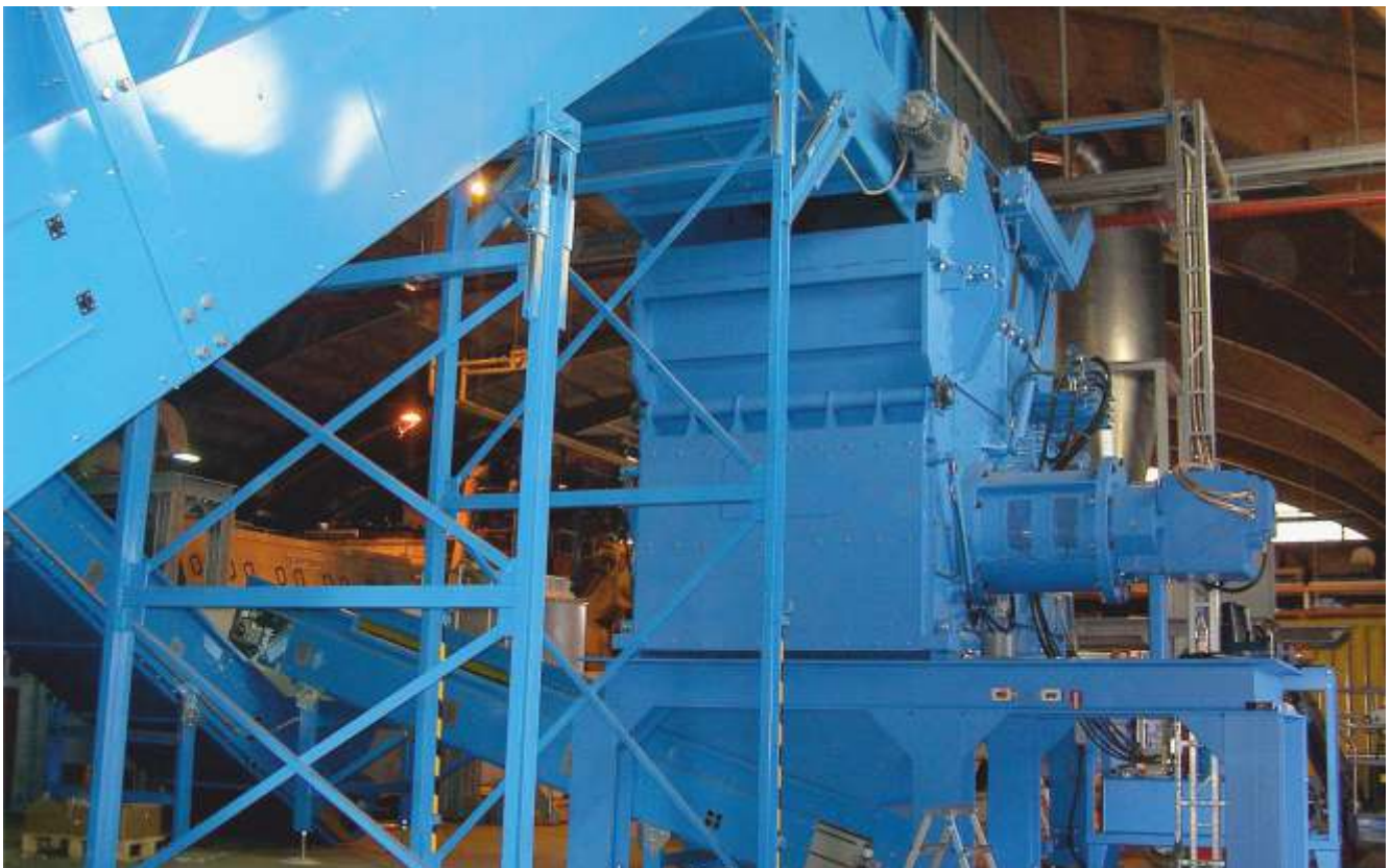
Shredder PowerLine WPL 2500 with direct drive, Cedo (Netherlands)
