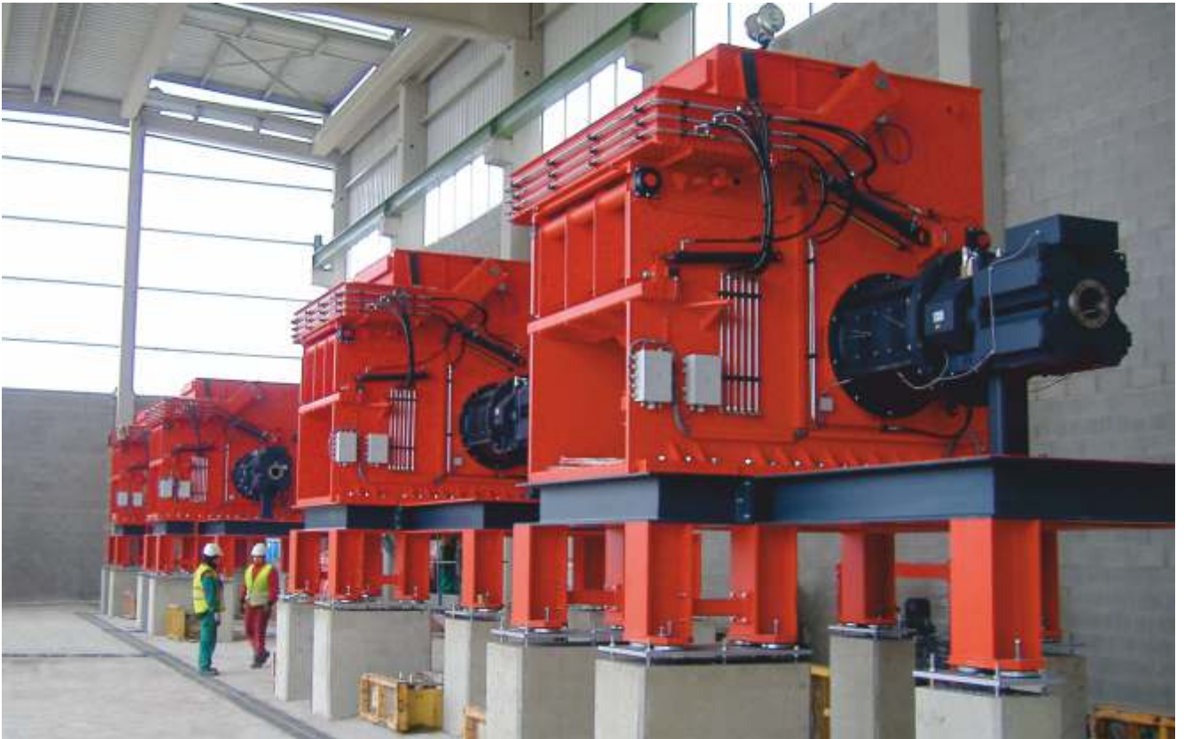
Shredder PowerLine with direct drive Saica (Spain)
