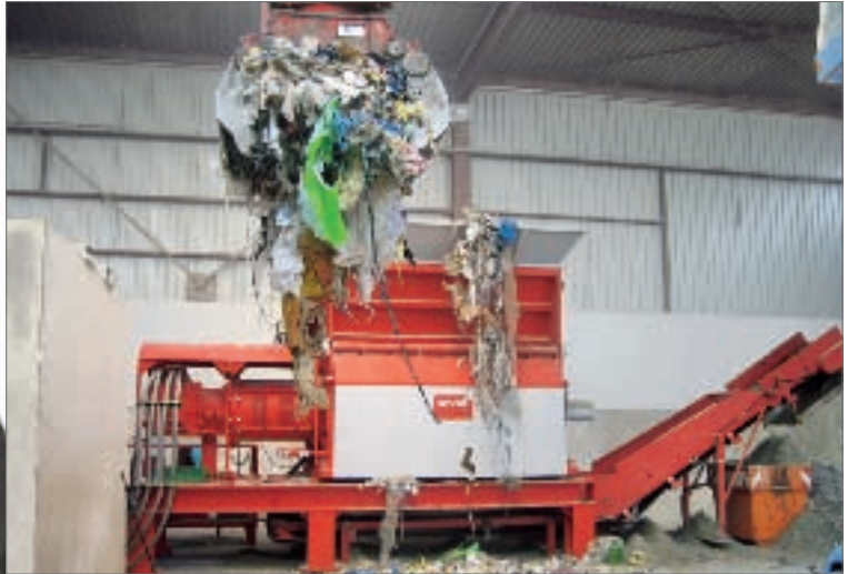
Strong in picking up: a gripper is used to feed PreCut.
