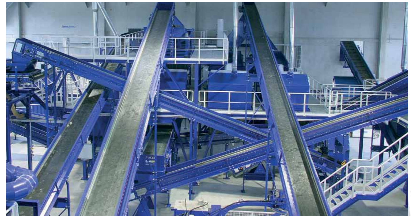
54 conveyors interlaced in a complex system with different length, width, velocity.
