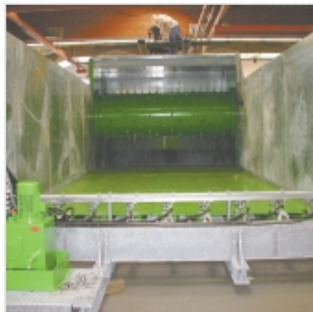
Push floors in all dimensions and types, with dosing unit or accessible by trucks. Our push floors are user-friendly with low maintenance and wear.
