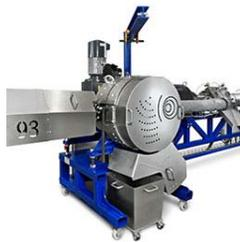
To ensure the disk filter does not clog up in continuous operation, a scraper removes the contamination from the surface of the rotating screen disc, which is discharged continuously from the CDF, while the filtrated melt is forwarded to the pelletizing system.
