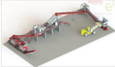
*This model of a proposed refuse-derived fuel (RDF) preparation system demonstrates the considerable number of steps that can be involved. (Illustration courtesy of eFactor3.)*
