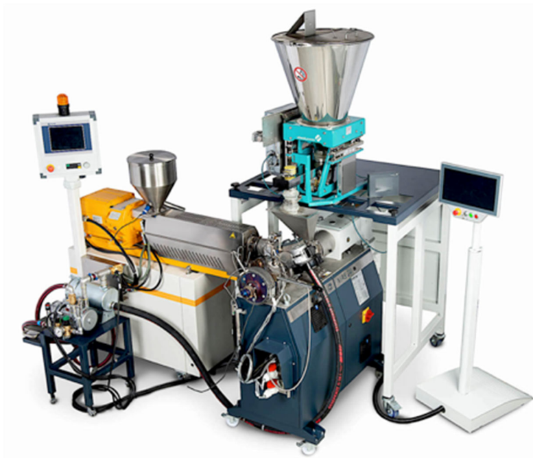
Fig.1: The conical co-rotating twin-screw extruders are available in 6 size stages with a throughput ranging from 10 to over 2,000 kg / h.
