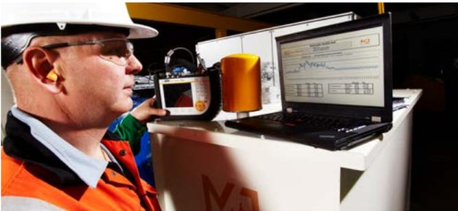
**Calculation of operations** Repairs and operational downtime can prove expensive if you simply wait for the shredder's wear parts to seize up. Our skilled service team can check all wear parts and can calculate their remaining service life. Then you will be aware when individual parts must be replaced, and how much this will cost. Calculation of operations ensures that wear parts are always replaced on time, so you experience the lowest downtime with the M&J shredder.
